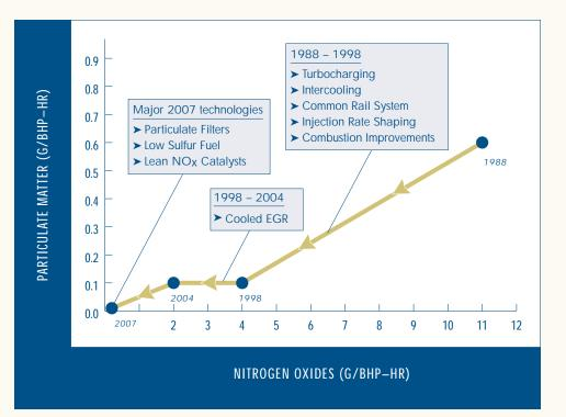
technology from Europe). Future emission reductions will be far more difficult, in part because catalysts and other emissionscontrol devices developed for gasoline engines are not transferable to diesels. Considerable effort is now being devoted to developing new diesel-specific technologies.
