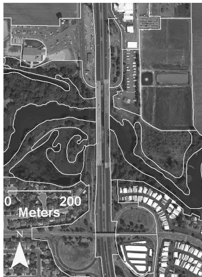
Fig. 4. Details that can be extracted from 1-foot black and white imagery used by the California Department of Transportation.
