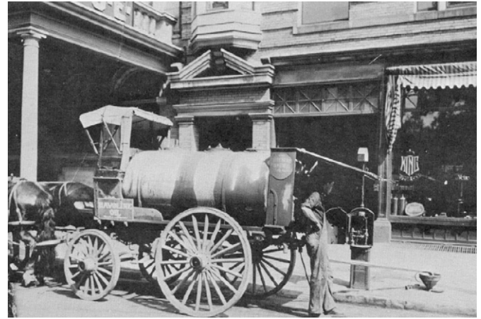
Fig. 6. A horse-drawn tank wagon refueling an early Bowser curb pump in front of a King automobile dealer (Milkues, 1978, p. 82).
