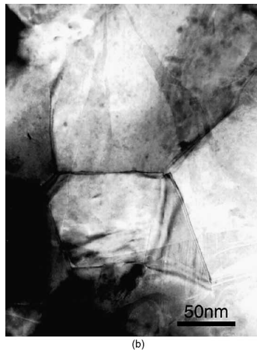
Fig. 4. TEM micrograph of the FAST sintered Ni samples at temperature 520 °C and heating rate (a) 90 °C/min, (b) 210 °C/min.
