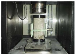
A comprehensive laboratory study to compare flexural and compressive strength, free shrinkage, coefficient of thermal expansion, and elastic modulus was undertaken on six concrete mixes typical of those used, or considered for use, by Caltrans in LLPRS.
