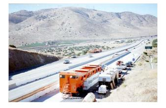
The Heavy Vehicle Simulator (HVS) testing program was initiated with a pilot study at the UCPRC Richmond Field Station. This included the evaluation of various types of instruments, methods of data recording, and the logistics involved with placing concrete around sensitive instrumentation. After the slab was cast, the HVS was used to evaluate performance of the various instruments as well as the performance of the slab under
