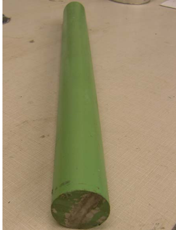
Figure 2.4. Epoxy-coated steel dowel.
