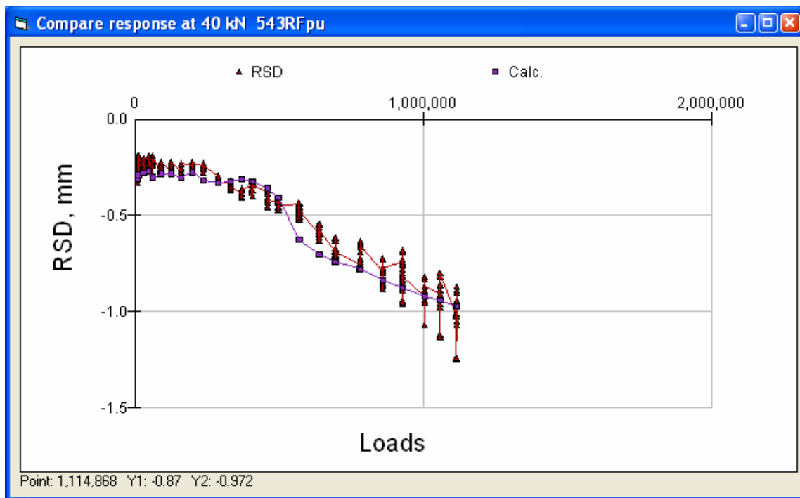
Figure 177. Section 543RF Road Surface Deflectometer, at 40 kN.
