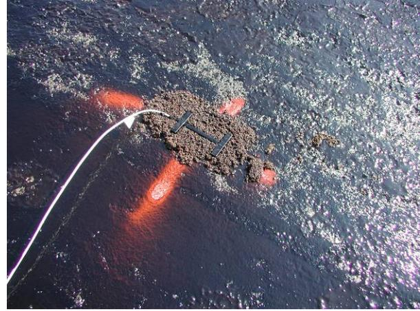
**Figure 2.12: Installation of strain gauges**
