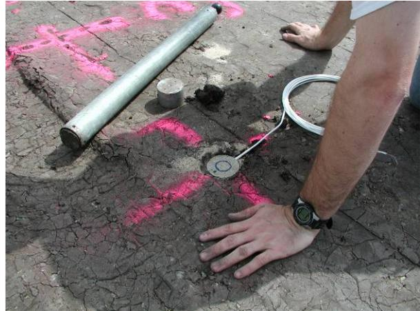
**Figure 2.9: Installation of pressure cell**
