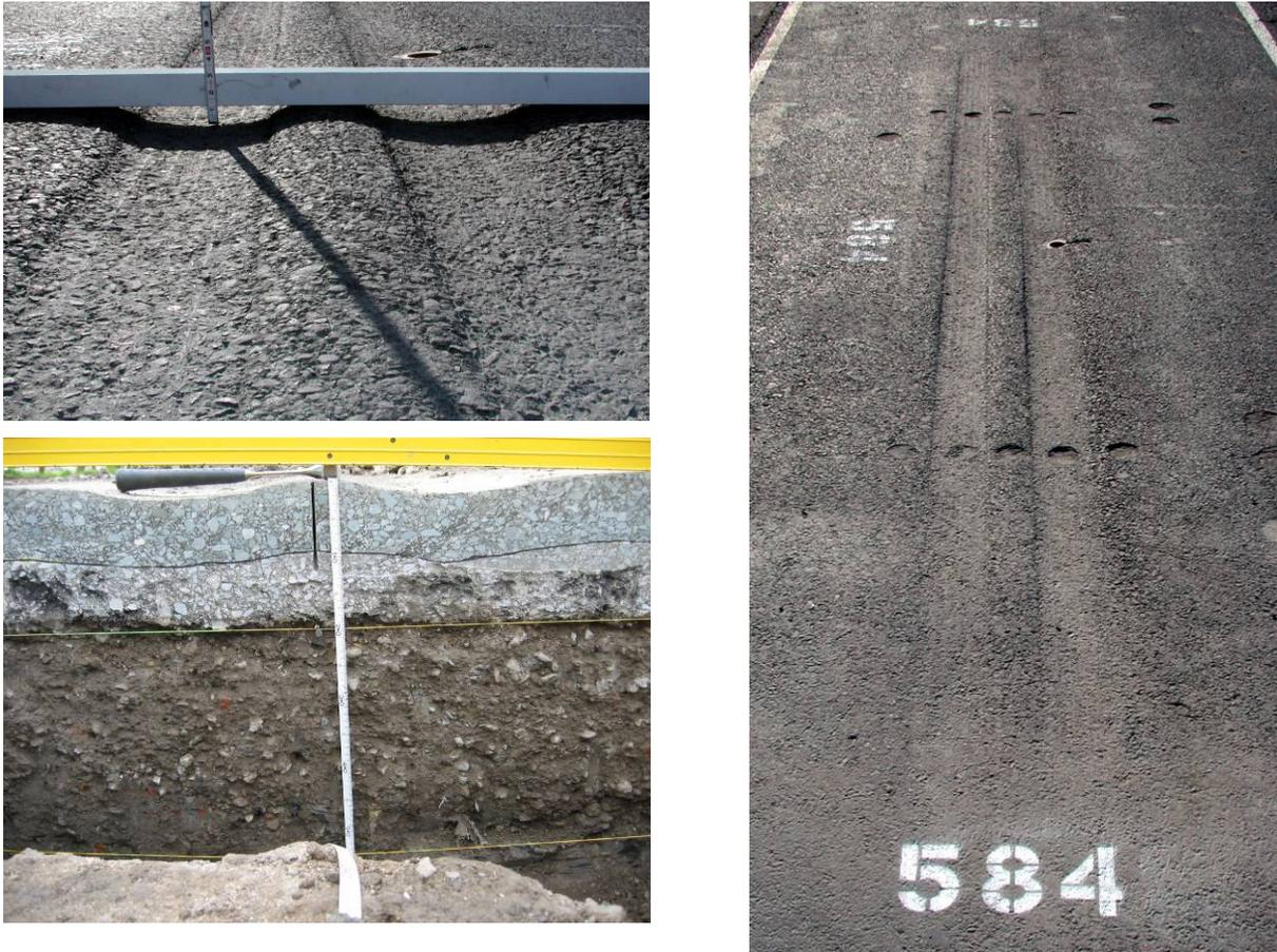
Figure 3.57: 584RF: Section photographs at the end of the test.
