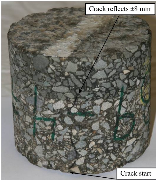
Figure 3.74: 45 mm MB4-G: Cracks on core.
