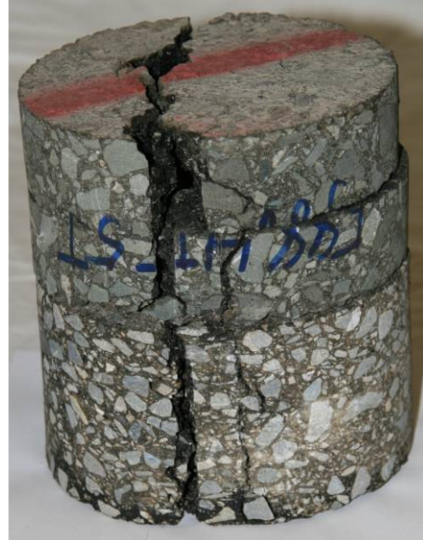
Figure 3.73: AR4000-D: Cracks on core.
