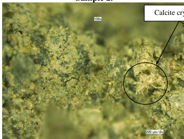
Figure 3.82: Optical microscope view ( \pm 100\times ) of calcite crystal development associated with cracks.
