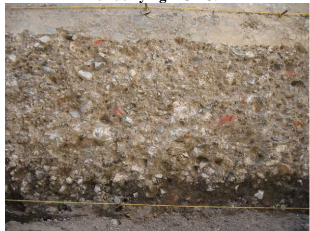
Figure 3.49: 588RF#4 areas of strong base cementation.
