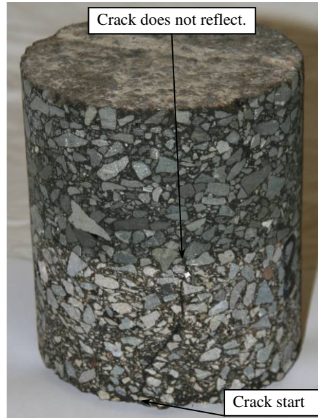
Figure 3.75: 90 mm MB4-G: Cracks on core..
