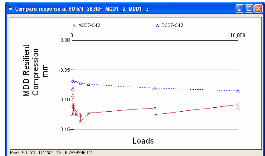
Figure B.20: 583RF, measured and calculated resilient compression of lower AB layers.
