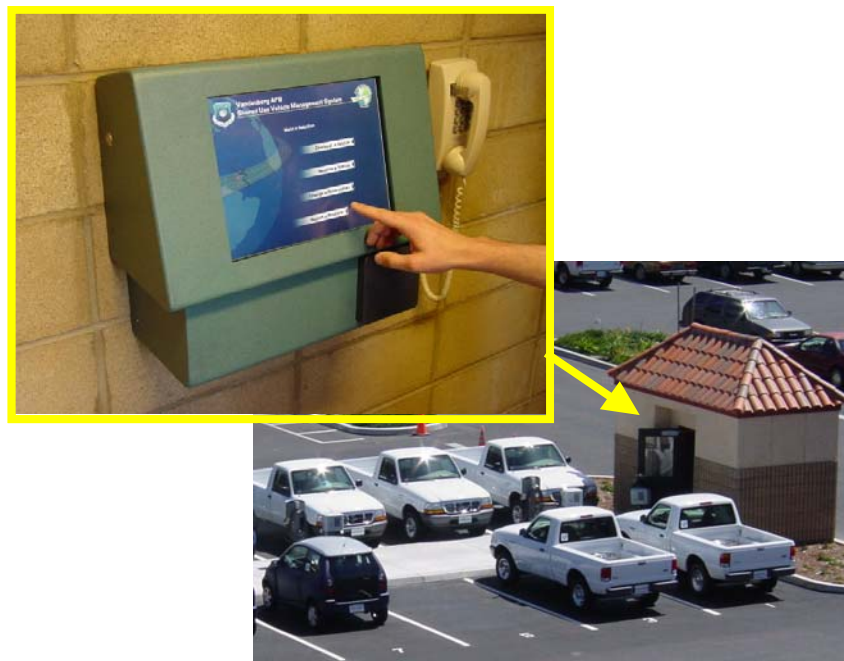
Figure 3.6. Touchscreen kiosk terminal (located inside small building) used to check-out shared-use vehicles (electric pickups and electric city cars).
