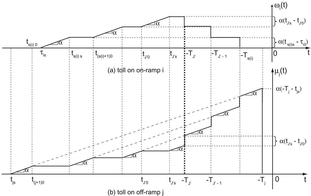
Fig. 11. The optimal dynamic toll on the ramps.
