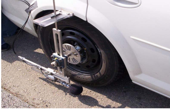
Figure 3: On-board sound intensity (OBSI) microphone setup.
