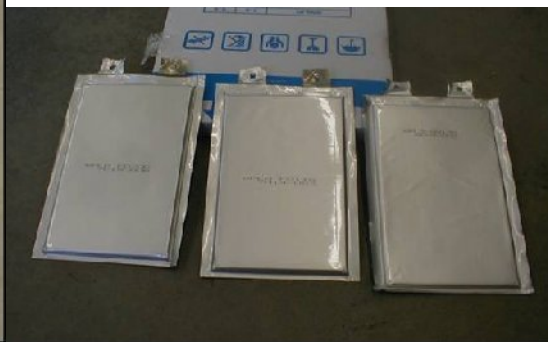
Figure 1: Small, spiral wound cells Figure 2: Pouch packaged cells
