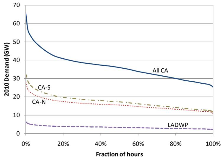
Figure 21. Load duration curve used in 2010 dispatch modeling.
