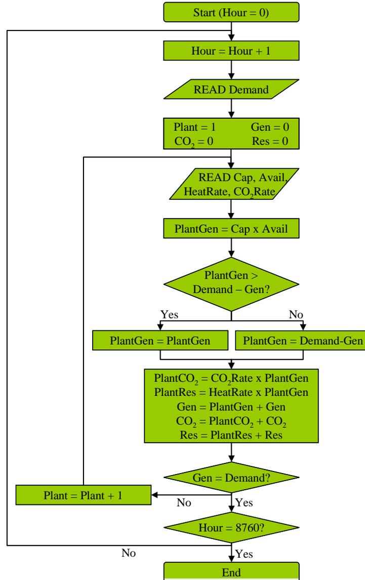
Figure 25. Flow chart of logic in the EDGE-CA model.
