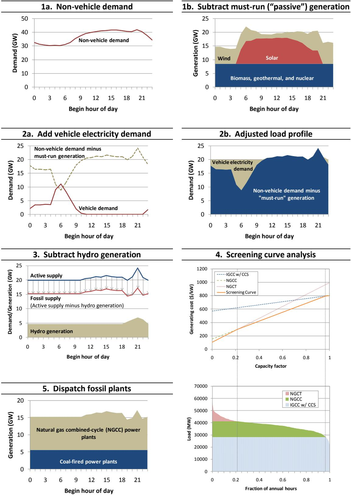
Figure 48. Framework of LEDGE-CA model for long-term electricity supply analysis.
