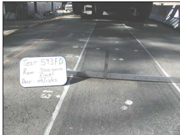
(b) End of test after 300,000 repetitions
