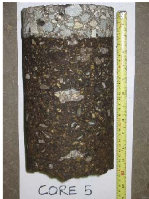
Figure 4.40: 150 mm core taken from the southbound lane.
