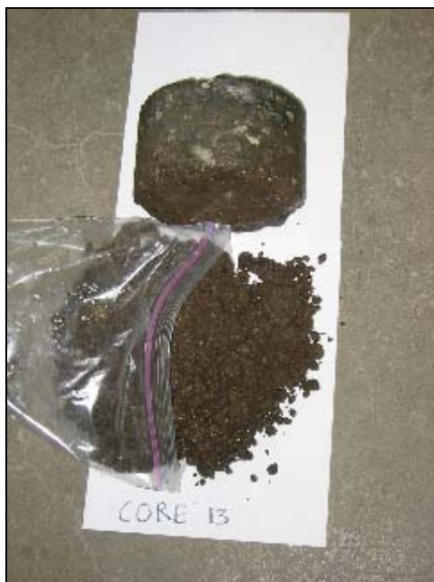
(a) Core 13 taken from the HVS test section
