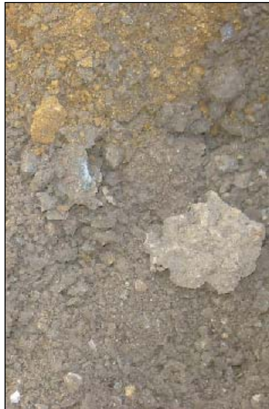
(b) The material below the base layer broke out in flaky pieces
