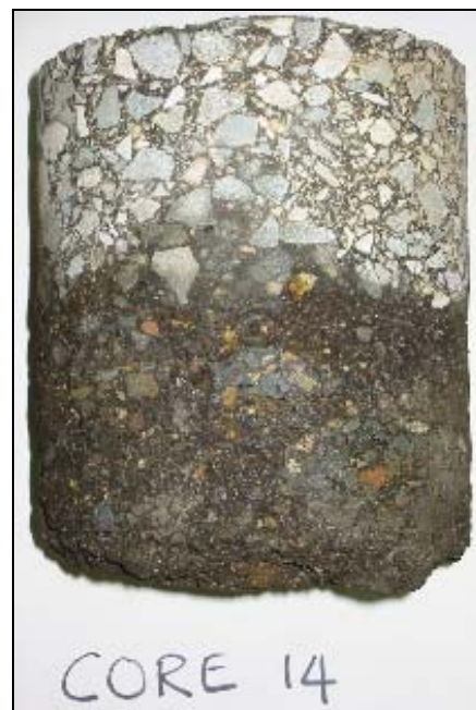
(b) Core 14 taken next to the HVS test section
