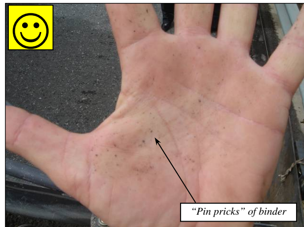
Figure 6.31: Asphalt binder dispersion check (good).
