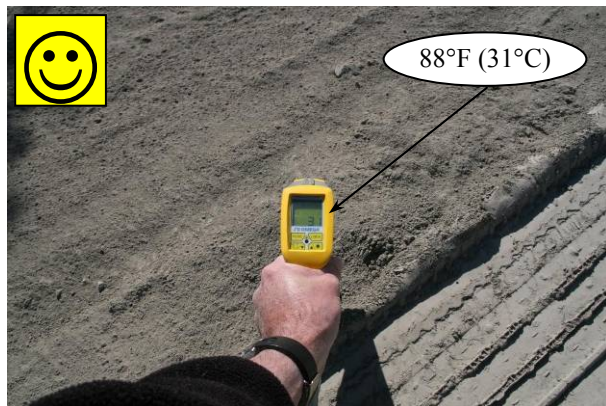
Figure 6.22: Portland cement temperature prior to recycling (warm).
