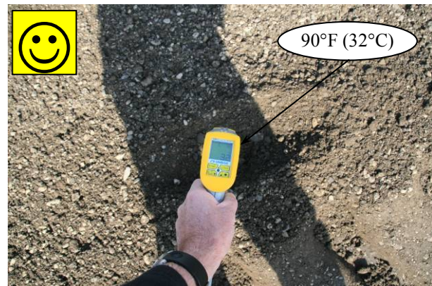
Figure 6.23: Recycled material (warm, good dispersion).
