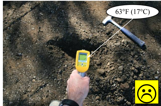
Figure 6.21: Recycled material (cold, poor dispersion).
