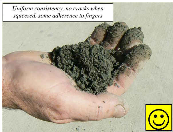
Figure 6.30: Moisture content checks (good).
