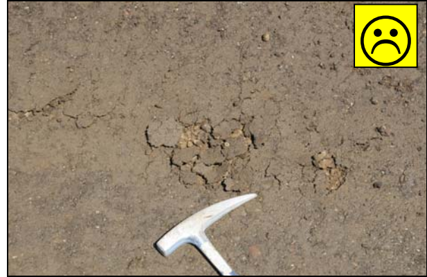
Figure 6.45: Laminations after grading.
