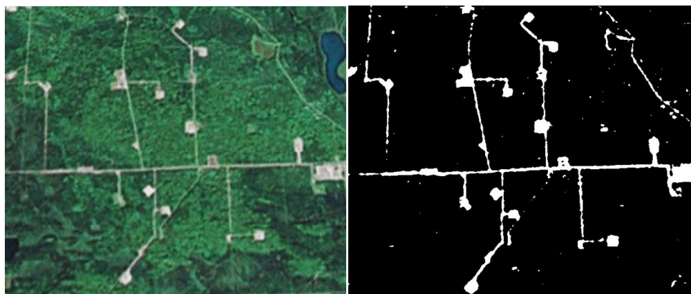
Figure S1. A. Image analysis of land disturbance for California Elk Hills oil field. Left: images extracted from Google Earth and attributed to Telemetrics, TeleAtlas and Digital Globe 2009. Right: Converted black and white image to estimate the percent of disturbance (white area). B. Illustrative image analysis of land disturbance for Alberta oil field. Left: images extracted from Google Earth and attributed to Telemetrics, TeleAtlas and Digital Globe 2009. Right: Converted black and white image to estimate the percent of disturbance (white area).
