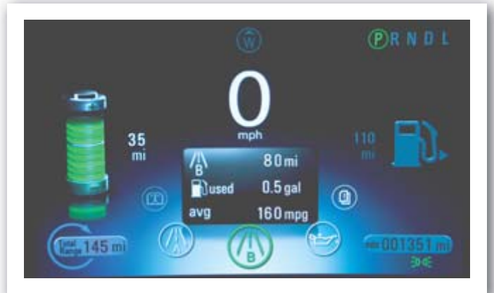
The Chevrolet VOLT dashboard display provides real-time energy consumption information to the driver
