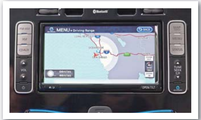
The GPS on the Nissan LEAF constantly updates the driving range on current state of charge
