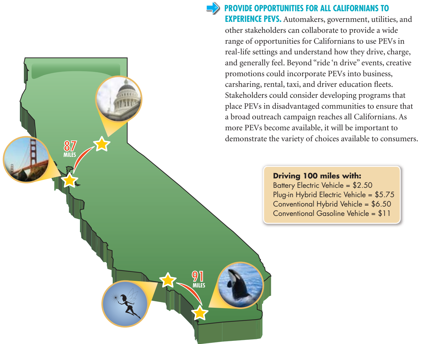
Figure 5. PEVs can cut fuel costs by 80%. PEV fuel savings are an important consumer benefit that should be part of public outreach messaging. Analysis assumes a gasoline price of $3/gallon, electricity price of $0.10/kWh, and a plug-in hybrid electric vehicle with 20 miles all-electric range (see Chapter 6).
