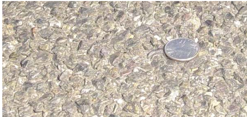
Figure 2.1. The Open Graded Asphalt Concrete on the I-80 test section. The diameter of the US quarter dollar coin is 24 mm.
