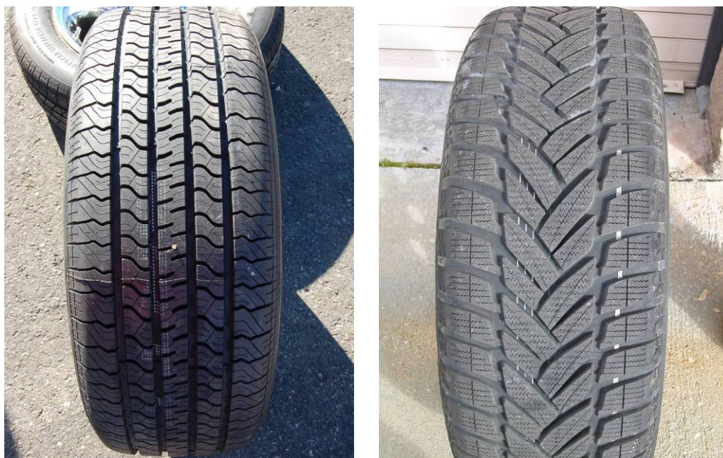
Figure 1.8. A Standard Reference Test Tire (SRTT) to the left (photo Bruce Rymer, Caltrans) and the Dunlop SP Winter Sports tire to the right (photo Paul A. Donovan, Illingworth & Rodkin, Inc).
