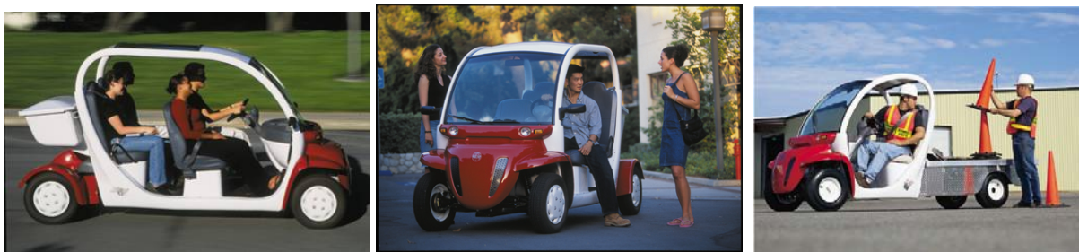
Figure 2.1. a) A four-seat neighborhood electric vehicle; b) a two-seat NEV; and c) a utility NEV.
