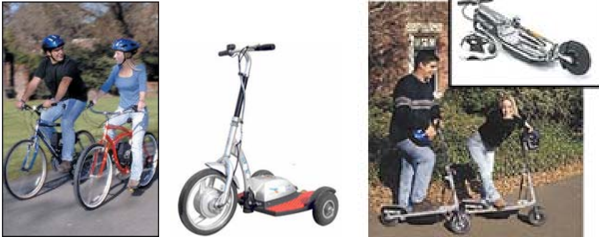
Figure 2.2. a) electric bicycle; b) electric 3-wheel scooter; and c) electric 2-wheel scooter.
