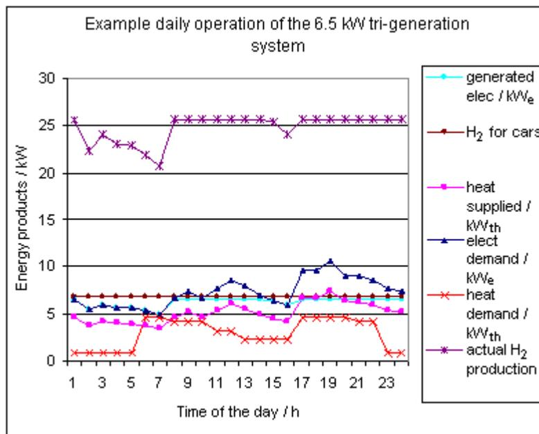
Fig. 6.4 Daily operation of a 6.5 kW tri-generation system
