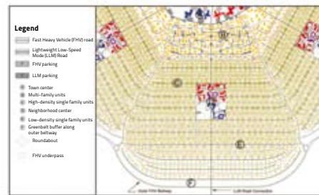
(Below left) Figure 1 shows plan of dual road system for new towns, with land uses (Below right) Figure 2 shows plan of neighborhood branch (Bottom left) Figure 3 shows details of driveways and residential street (Bottom right) Figure 4 shows the town center
