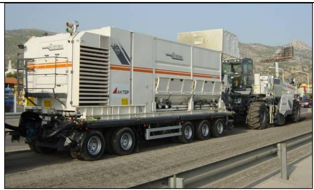
(b) Rotary mixer/recycler coupled to slurry applicator
