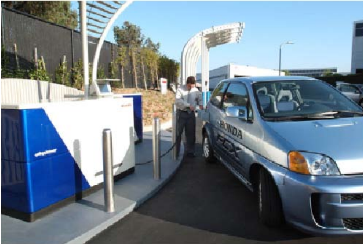
Figure 5: Demonstration of the Honda/Plug Power Home Energy Station
