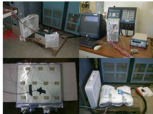
Figure 2: Testing of the 50 Ah lithium titanate oxide cell
