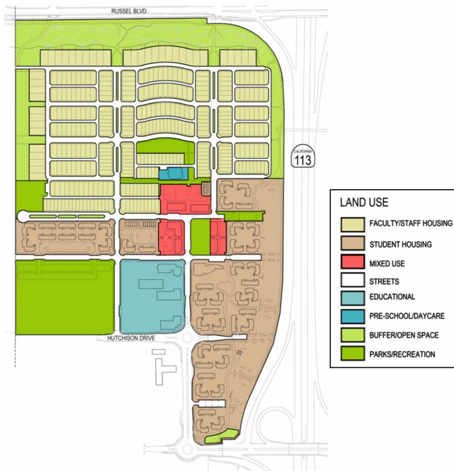
Figure 1. West Village site plan. The east–west orientation of streets and buildings in West Village makes possible passive solar orientation of buildings. Source: Carmel Partners, UC Davis Office of Campus Planning and Community Resources.
