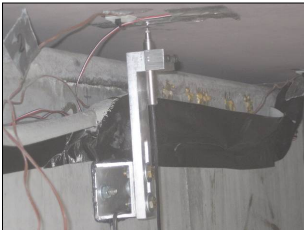
Figure 3.12: LVDT, strain gauge, and thermocouple on midpoint under steel plate. (Instruments #7, #11, and #15)
