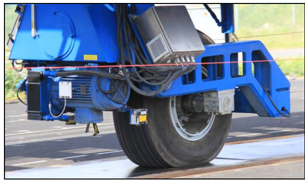
Figure 3.15: Aircraft tire (Boeing 737) configuration.
