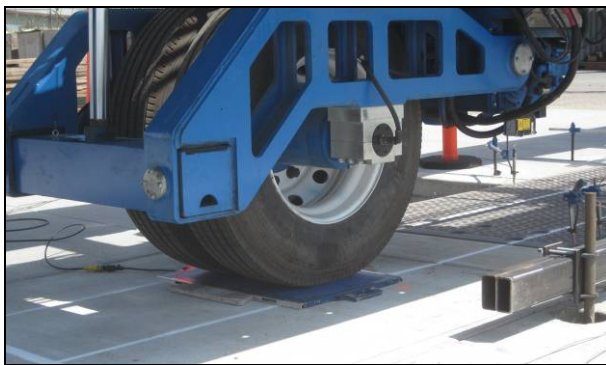
Figure 3.14: Dual truck tire configuration (note load calibration pad).
