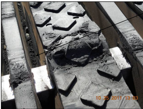
Figure 4.68: Phase 3.3: Tearing of rubber and accumulation of rubber particles in Trelleborg unit.
