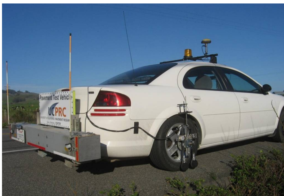
Figure 2.1: Instrumented vehicle with one set of sound intensity microphones on each side of the tire and an inertial profilometer with spot lasers, including a high-speed spot laser in the right wheelpath.
