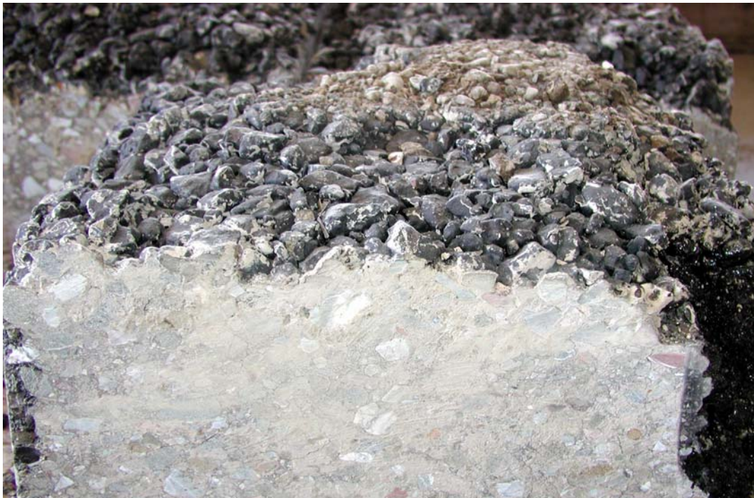
Figure 40b. ATPB slab from another HVS test section demonstrating appearance of ATPB without fines infiltration.
