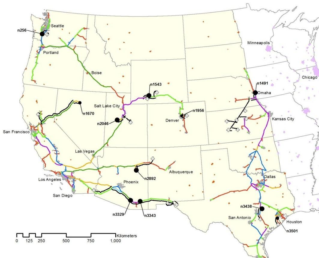
Figure 30: Optimal infrastructure design for tranche 3 (H<sub>2</sub> Partial Success scenario)
