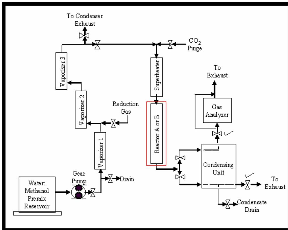
Figure 2: Schematic of HYPALU reformer/reactor system [2]
