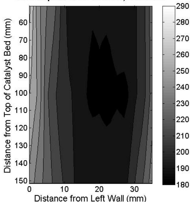
Figures #4-5 Radial temperature profile charts for the Low Aspect ratio Reactor at 5 and 20 ml per minute flow rates (corresponding to a GHSV of 1 and 4 respectively)
