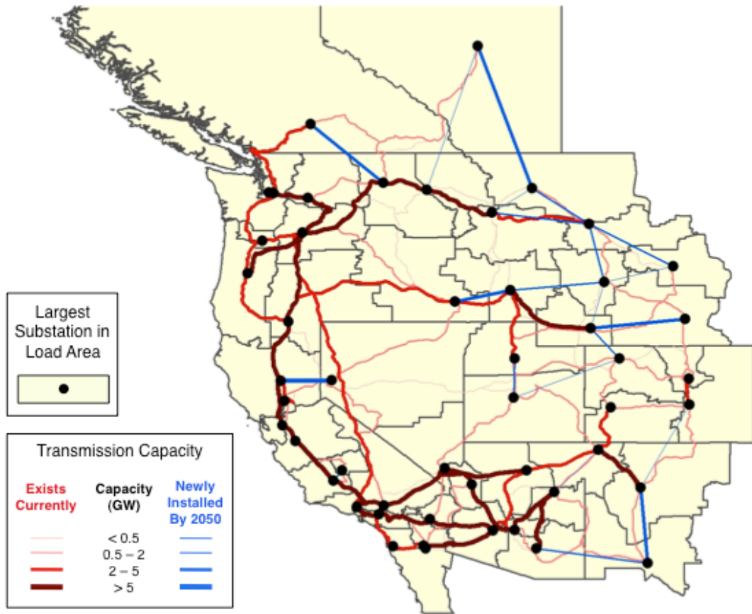
Figure S66: Existing and new transmission capacity between load areas in 2050 for the Base Case scenario. New transmission is built along existing transmission corridors when possible, but is depicted here with straight lines for clarity. Note the addition of large amounts of new transmission capacity to bring predominantly solar power from Northern Nevada into the Central Valley and San Francisco Bay Area regions of Northern California. Also, note the new transmission additions in the upper right of this map that bring Rocky Mountain wind west.
