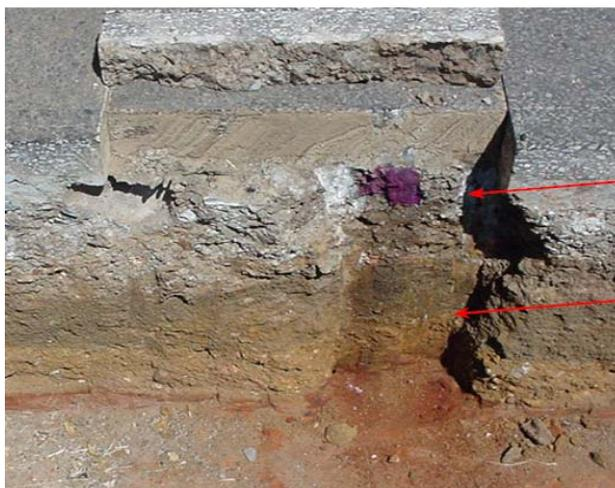
**Figure 3.14: Phenolphthalein reaction on base.**
