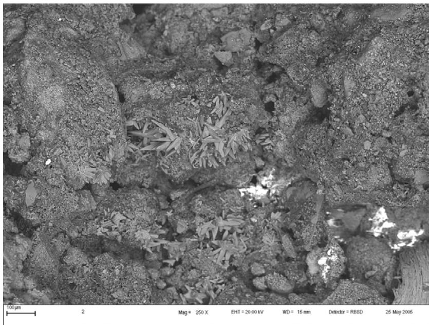
**Figure 3.16: Development of young calcite crystals associated with cracks.
