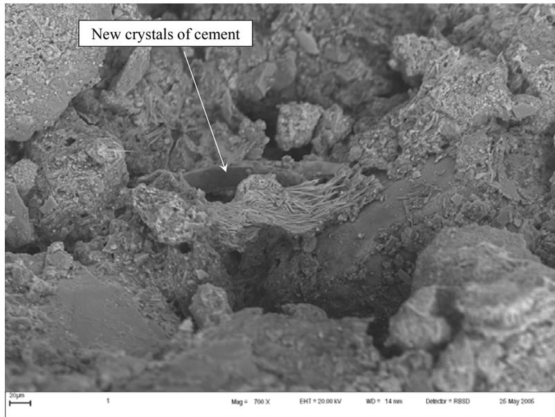
**Figure 2.1: New crystals of cement reaction products (10).**
