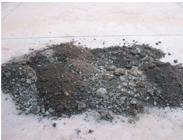
**Figure 3.13: Base course material from test pit.
