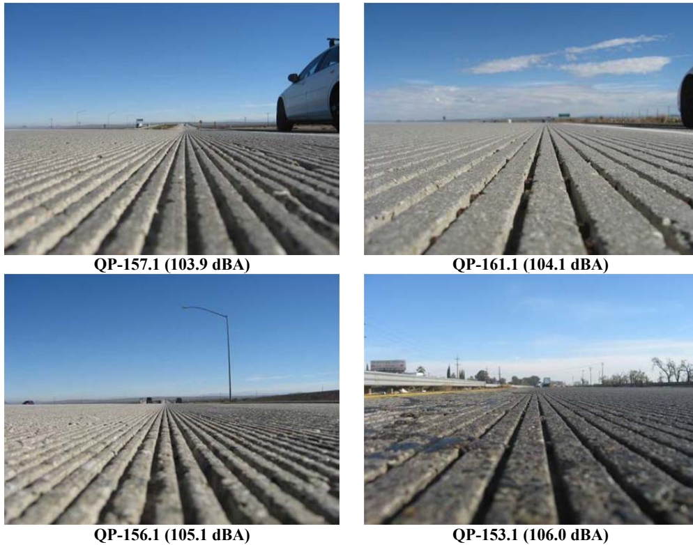
Figure 4.4: Example photographs of diamond-grooved surfaces and their OBSI levels.
