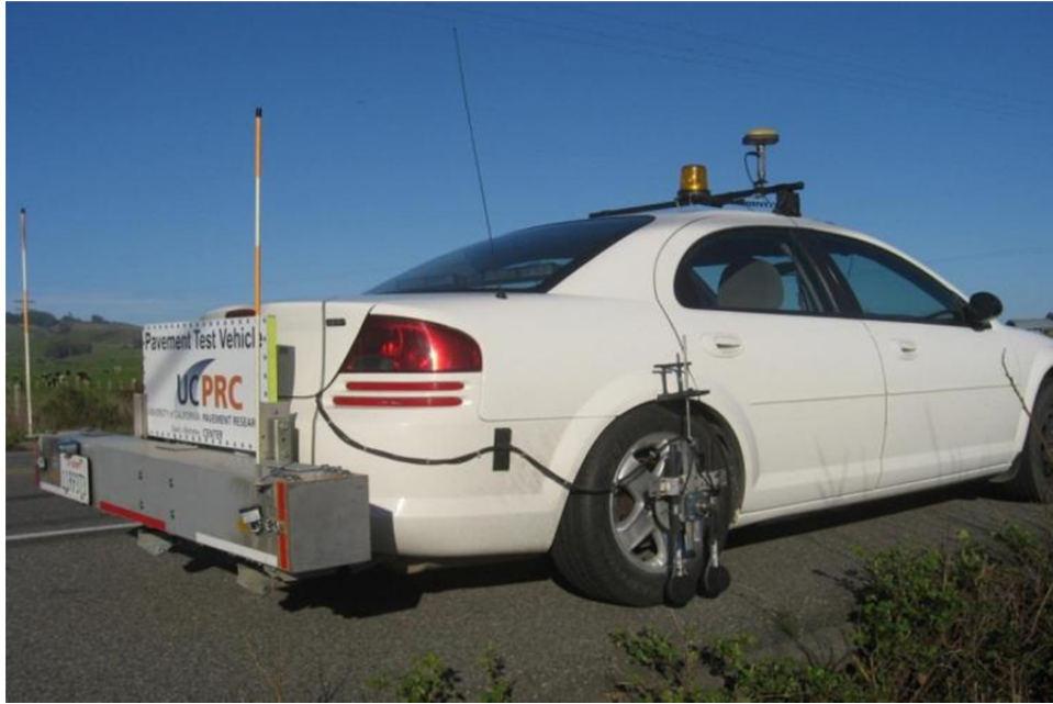
Figure 2.1: Instrumented vehicle with on-board sound intensity probes and an inertial profilometer.
