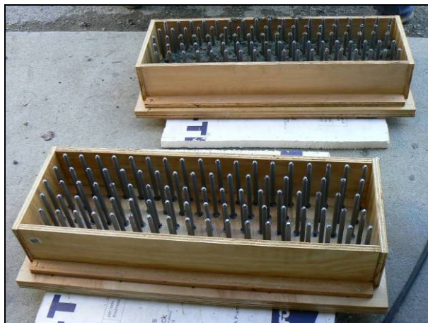
Figure 4.42: Cast beam specimen molds.
