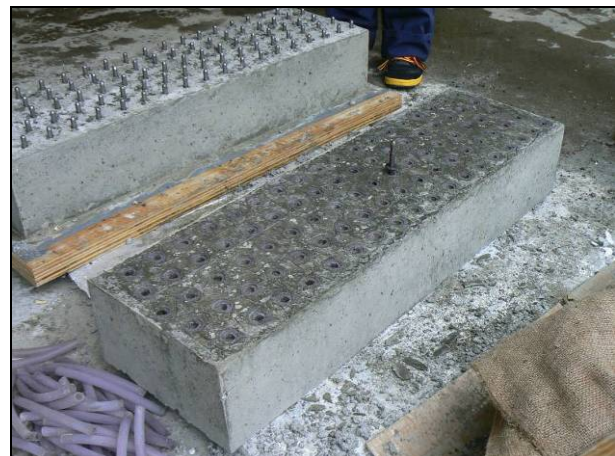
Figure 4.43: Demolded cast beam specimen.
