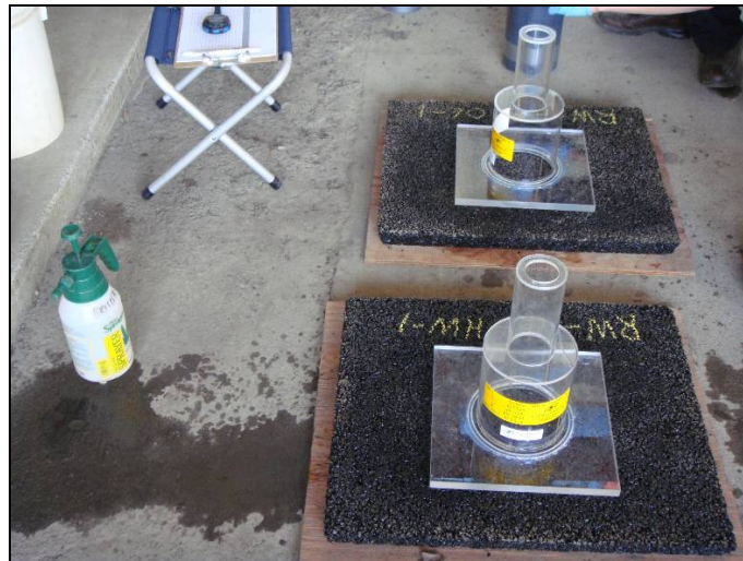
Figure 4.16: Permeability testing on compacted slabs.
