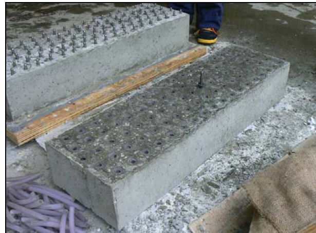
Figure 6.8: Demolded precast beam specimen.
