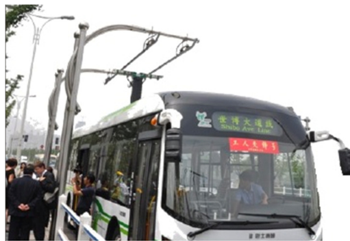
Overhead charging designs are already in use in China. One is shown above charging an ultra-capacitor
