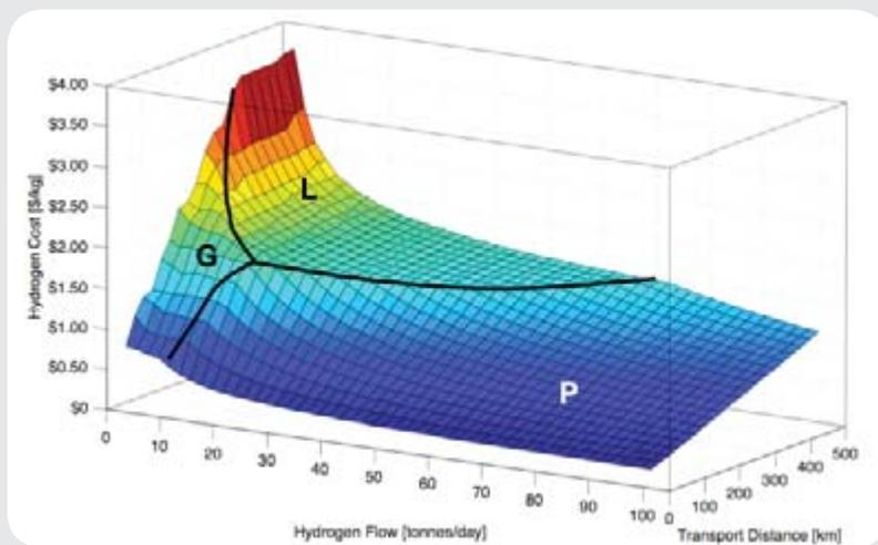
We compared three different hydrogen delivery modes to find the lowest-cost method. As hydrogen flow increases, delivery by hydrogen gas pipeline (P) starts to cost the least; as transport distance increases, liquid hydrogen trucks (L) win out. Compressed gas hydrogen trucks (G) cost least when both distance and flow are limited. Source: C. Yang and J. Ogden, “Determining the lowest-cost hydrogen delivery mode,” *International Journal of Hydrogen Energy* 32 (2007): 268–86.
