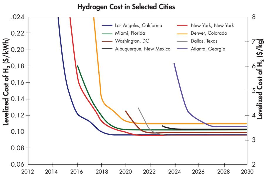
*The range and progression of delivered hydrogen costs over time is shown for selected “lighthouse” cities. Cost differences are due to phased introduction of hydrogen cars as well as to city size and density and local feedstock and energy prices.*
