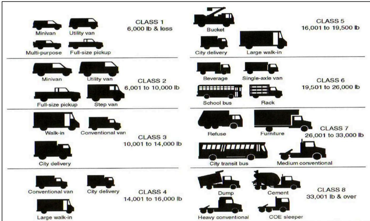
Figure 4-2: US commercial truck classification system (Eberhardt [195], page 9)
