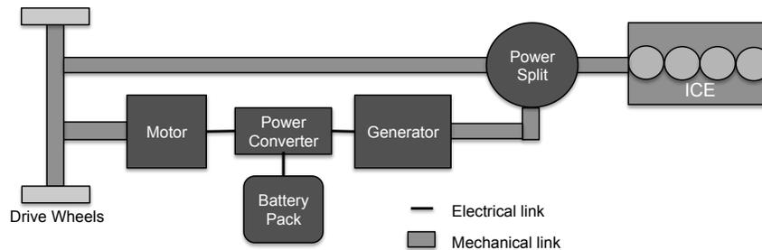
Figure 2-14: Series-parallel (power split) hybrid configuration
