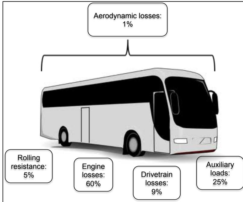
Figure 2-20: Example energy audit for half-seated 40-foot transit bus (32,000 lbs. GVWR) with air conditioning operating over the Central Business District cycle for 1 hour (created using data from Table 2-5 in [85])
