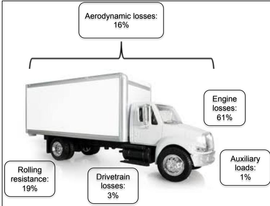
Figure 2-19: Example energy audit for a fully loaded (26,000 lbs. GVWR) MD truck vehicle operating on a level road at 40 miles per hour for 1 hour (created using data from Table 2-4 in [85])
