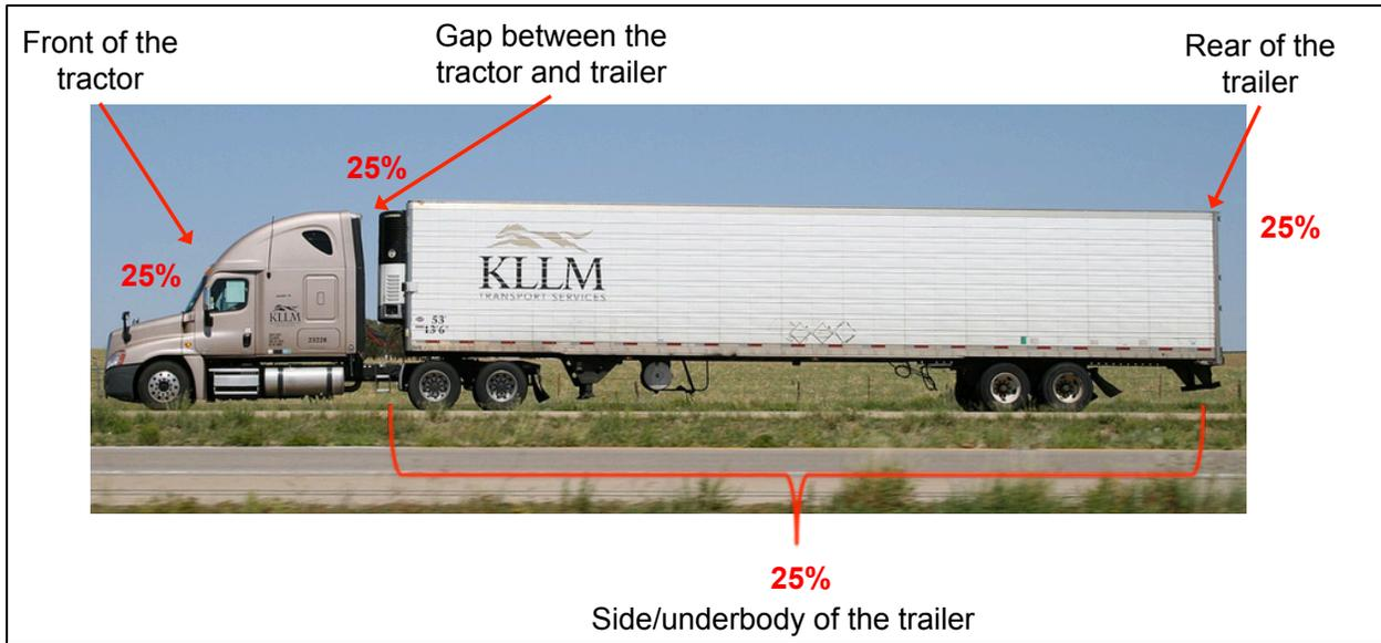
Figure 2-23: Four primary areas of aerodynamic drag on a tractor-trailer (adapted from [87])
