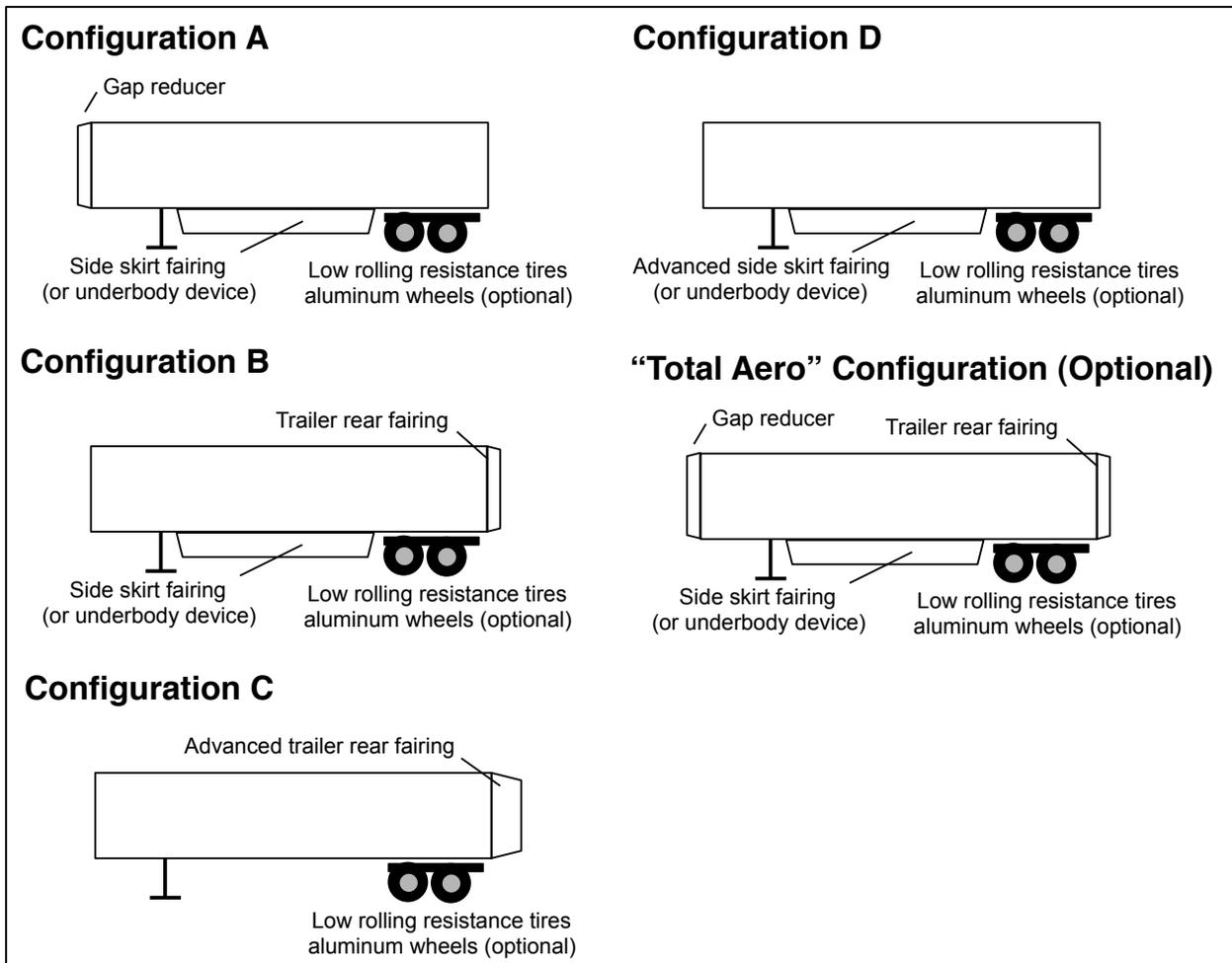
Figure 3-7: SmartWay certified trailer configurations (figures created using examples shown in [176])
