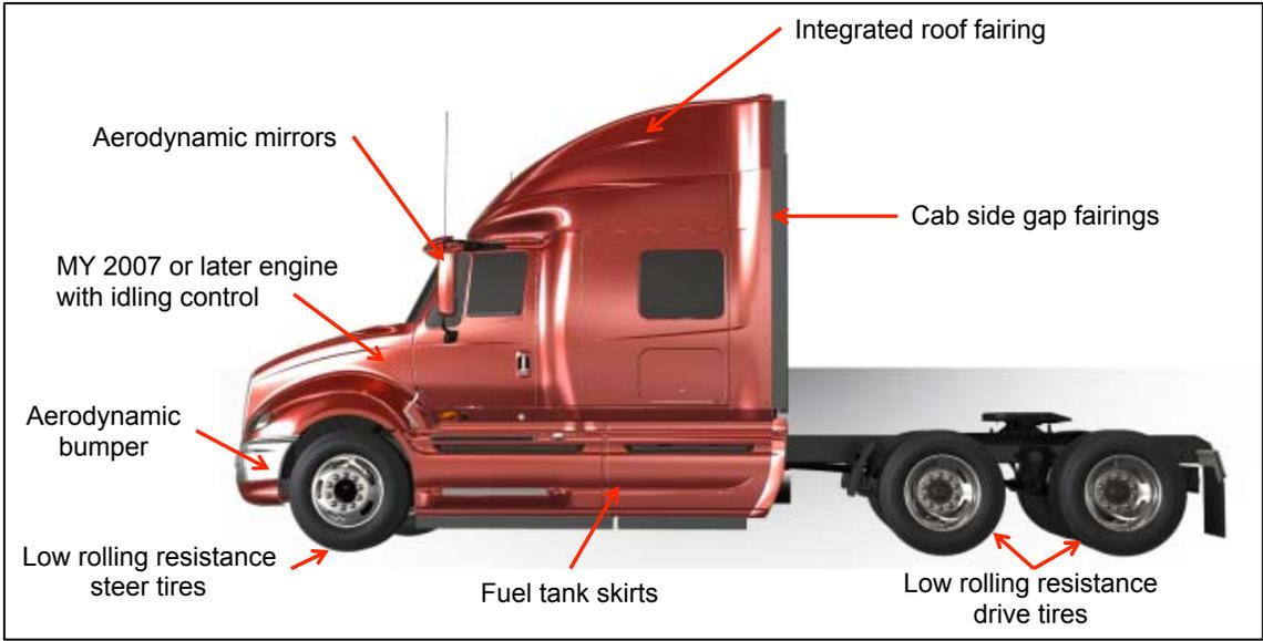
Figure 2-24: Example of a tractor with aerodynamic features<sup>8</sup>
