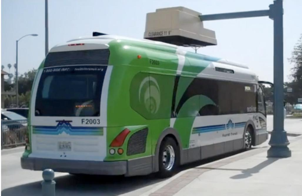
Figure 3-6: Foothill Transit's Ecoliner electric bus and its in-route fast-charging station [139]
