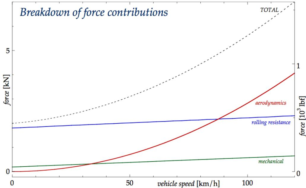
Figure 2-27: Drag forces as a function of vehicle speed for a tractor-trailer (Slide 23 in [90])
