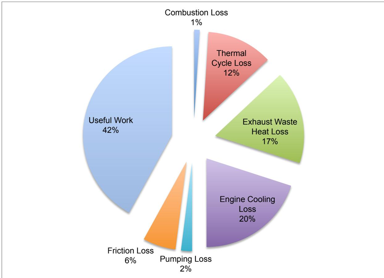
Figure 2-22: Example energy audit for a typical modern diesel engine (adapted from [86])
