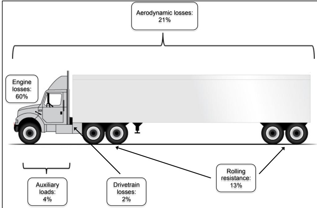
Figure 2-18: Example energy audit of a fully loaded (80,000 lbs. GVWR) tractor-trailer traveling at 65 mph (created using data from Table 3.1 in [84])
