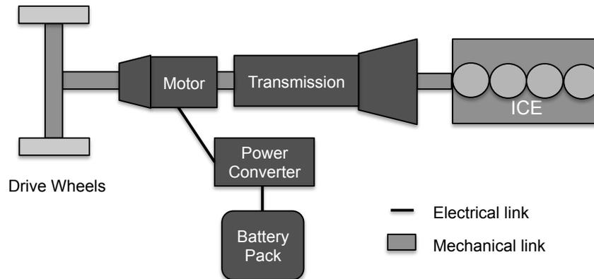
Figure 2-12: Post-transmission parallel hybrid configuration
