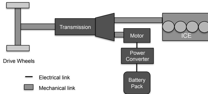
Figure 2-11: Pre-transmission parallel hybrid configuration
