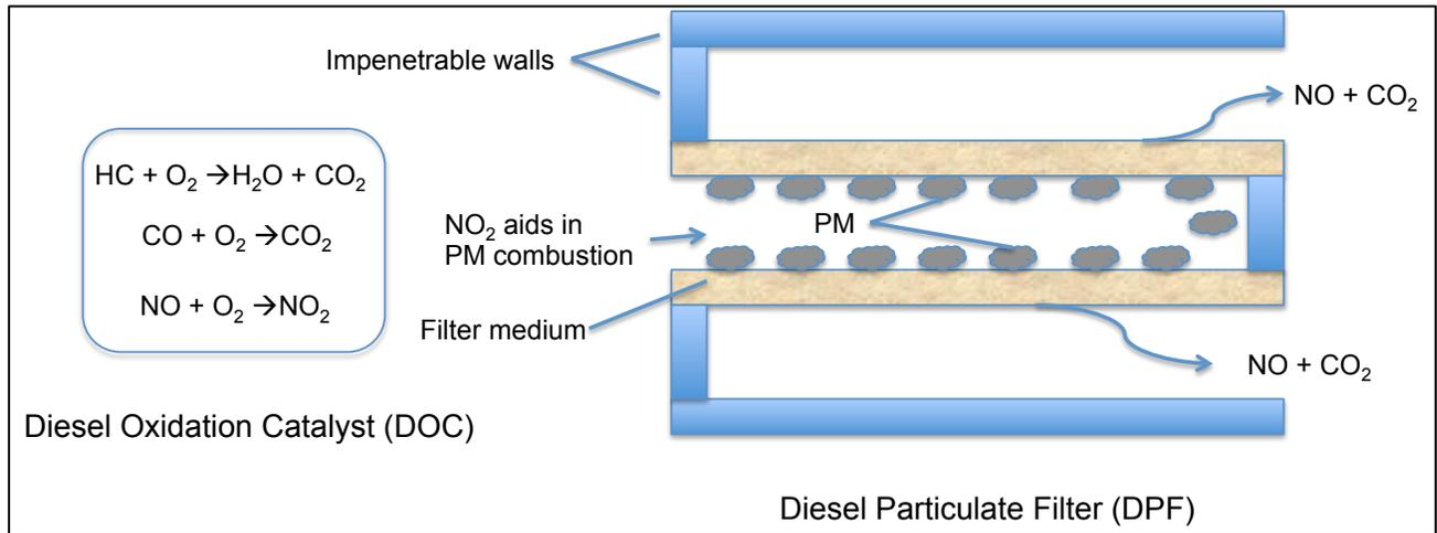
Figure 2-3: Operating principle of a diesel particulate filter
