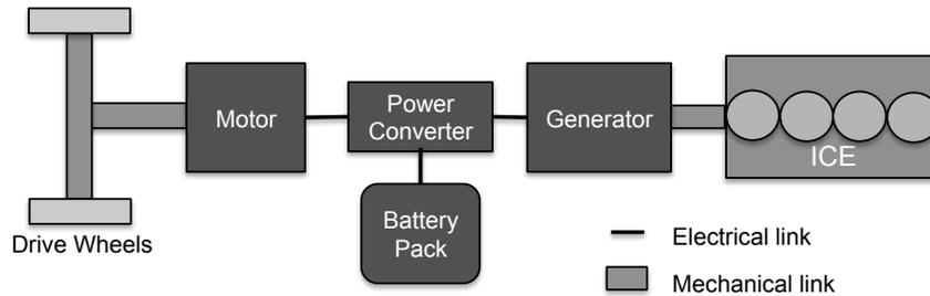
Figure 2-13: Series hybrid configuration
