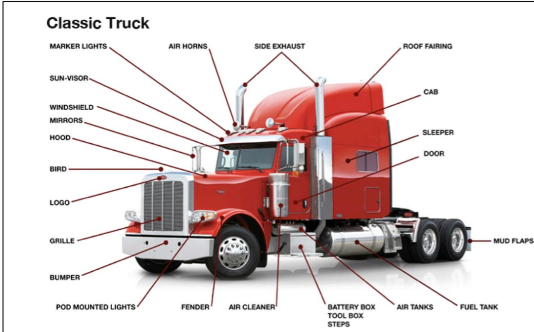
Figure 2-25: Example of a conventional or “classic” tractor<sup>9</sup>
