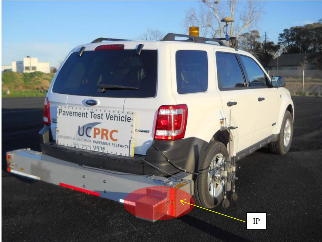
Figure 4.7: Instrumented vehicle with an inertial profiler (IP).
