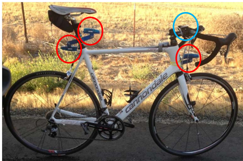
Figure 3.6: Bicycle instrumented with accelerometers (red circles) at three typical mounting locations and a GPS unit on the handle bar (blue circle).
