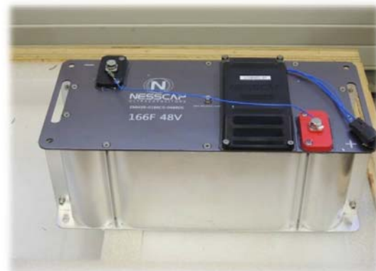
48V module (18 x 3000F cells)
