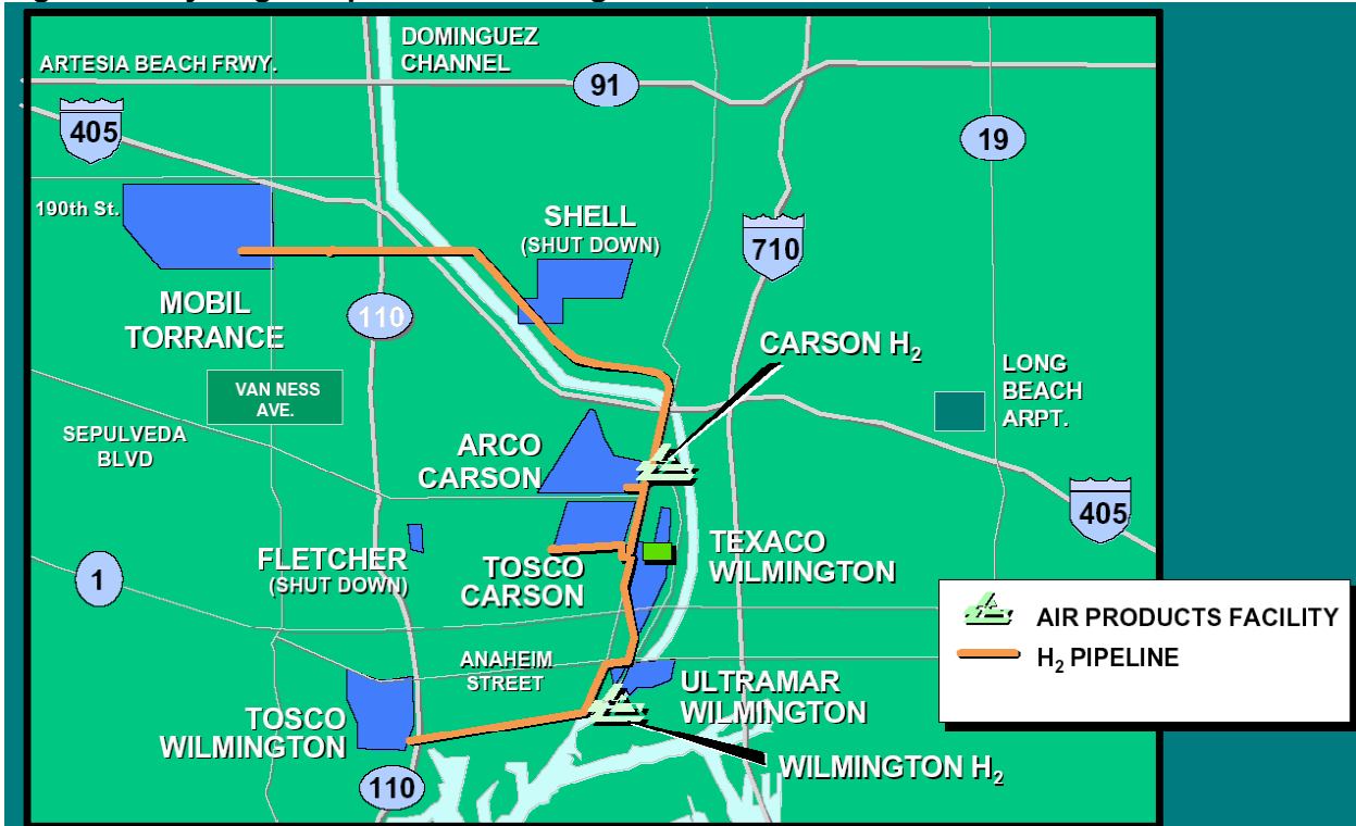
Figure 12: Hydrogen Pipeline in Los Angeles
