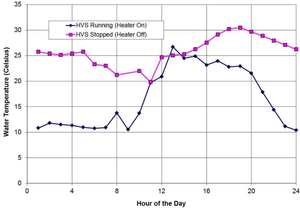
Figure 5.7: Average hourly water temperatures during HVS testing for Section 662HC grouped by HVS and heater status. (Section 662HC: dual wheel, Caltrans 3/8 inch mix with PG 76-22PM binder.)
