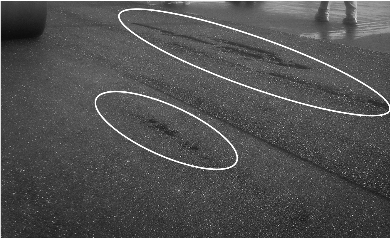
Figure 2.6: Scarring caused by crusted mix (Cell B1, #4P mix with PG 76-22PM).
