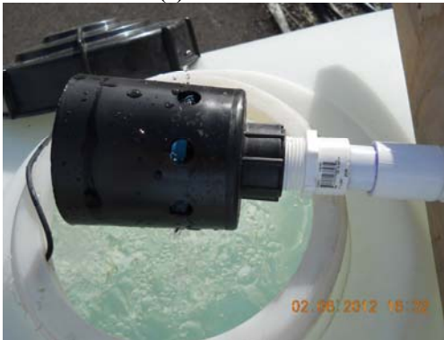
(b) Auto shut-off device to maintain constant water head
