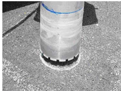
(k) Removal of cores for post-test scanning
