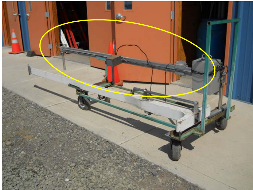
Figure 3.7: The laser profilometer.
