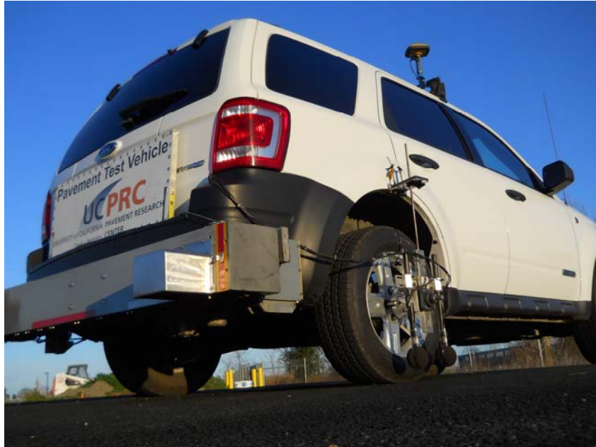
Figure 3.22: The UCPRC On-board Sound Intensity (OBSI) measurement vehicle.
