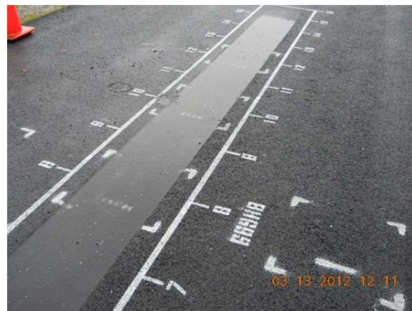
(b) Section 669HB: #4P mix with PG 76-22PM binder, OGFC thickness = 0.07 ft
