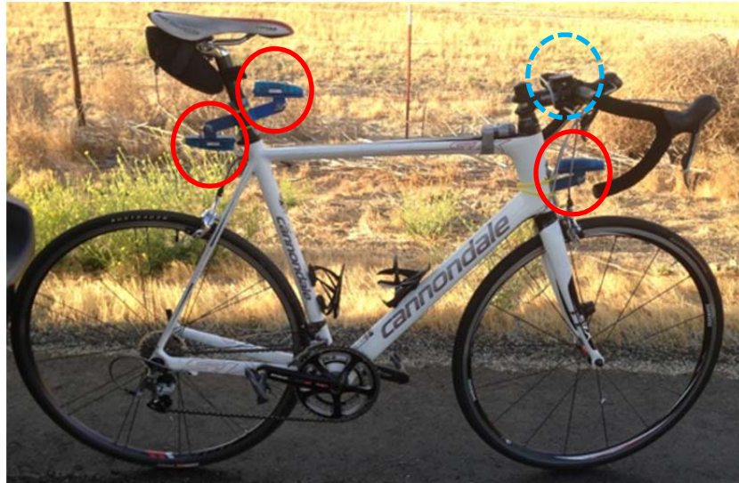
Figure 3.6: Bicycle instrumented with accelerometers (solid red circles) at three typical mounting locations and a GPS unit on the handle bar (circle of blue dashes).
