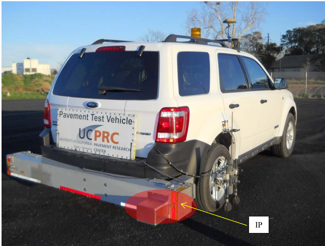
Figure 4.7: Instrumented vehicle with an inertial profiler (IP).
