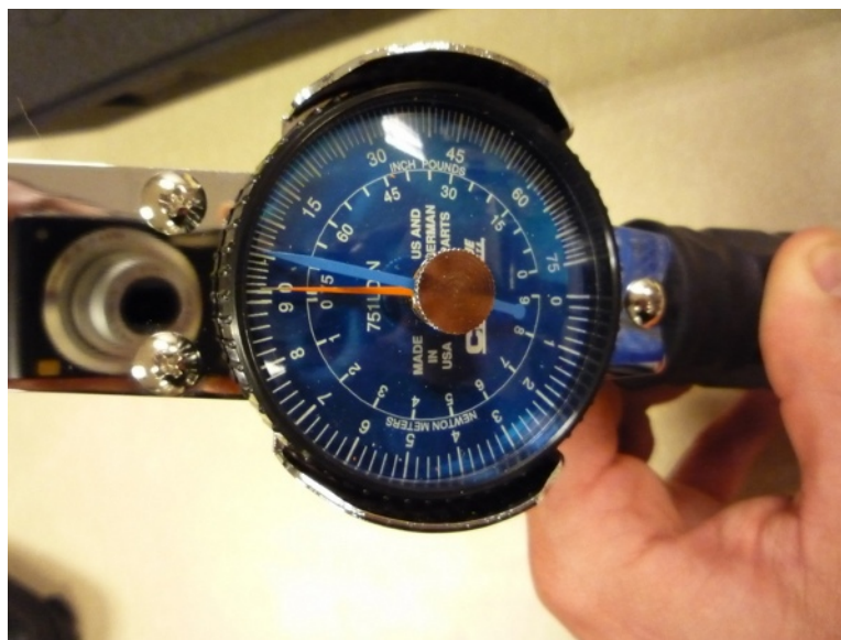
Figure 9.17: The dial indicator face of the torque wrench which reads out in inch pounds and newton meters.
