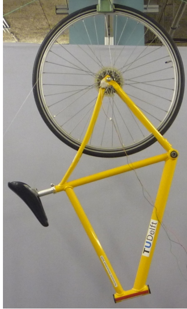
Figure 5.20: The yellow bicycle rear frame hung as a compound pendulum about the wheel axis (the wheel is fixed in place).
