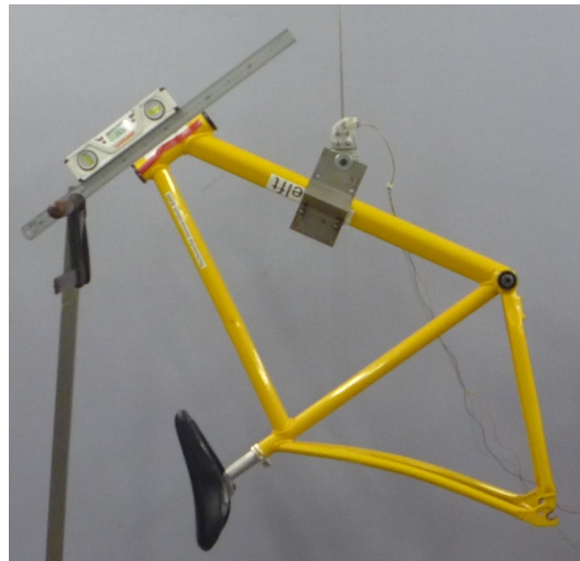
Figure 5.8: The digital level was mounted to a straight edge aligned with the head tube of the bicycle frame. This was done without allowing the straight edge to touch the frame. The frame was not absolutely stationary so this was difficult. The light frame oscillations could be damped out by submerging a low hanging area of the frame into a bucket of water to decrease the oscillation.
