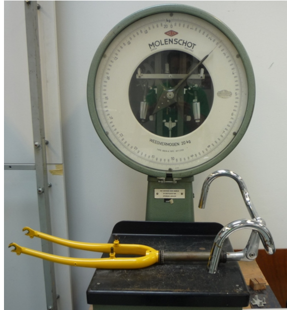
Figure 5.6: The scale used to measure the mass of each Delft bicycles' components.
