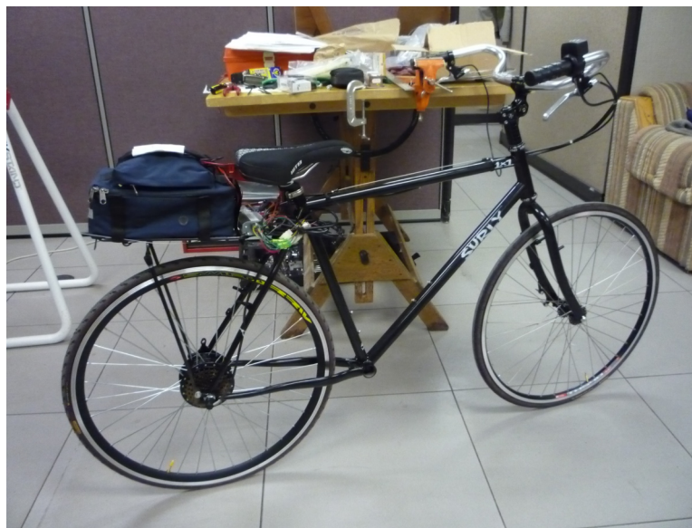
Figure 9.1: The Surly 1x1 with 700c wheels and basic handlebars for upright seating. An Amped Bikes geared hub motor is shown installed along with the lead acid battery kit on the rear rack.
