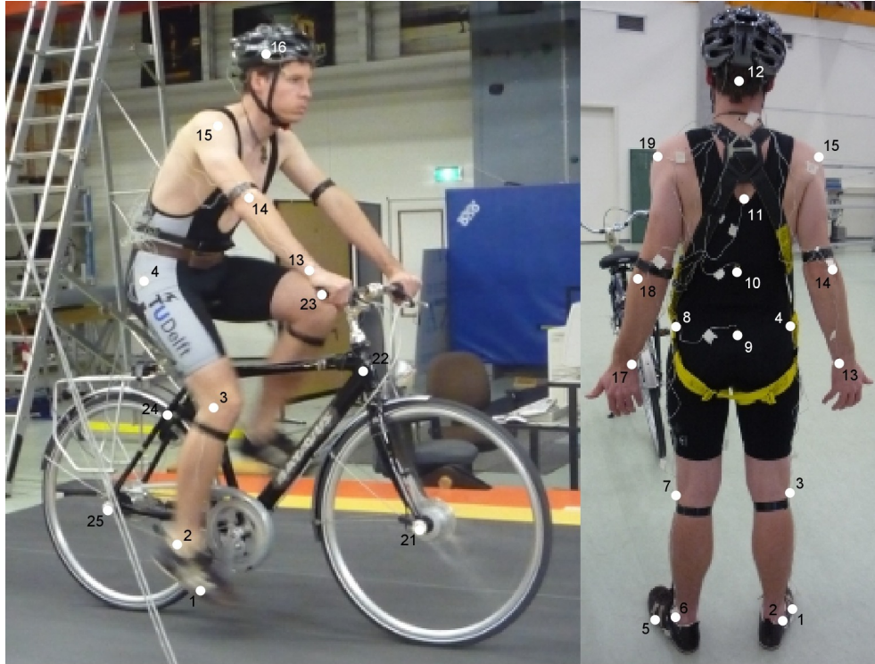
Figure 8.2: Rider 1 and the Batavus Stratos Deluxe with marker positions. Body marker positions visible from the rear.
