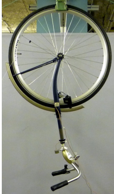
Figure 5.21: Browser fork hung as a compound pendulum.
