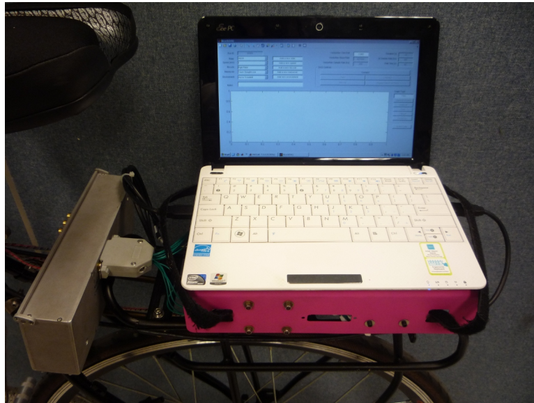
Figure 9.33: The laptop mounted to the rear rack.
