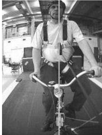
Figure 7.5: Video still of normal pedaling at low speed (5 km/h) showing large lateral (left) knee motion and (right) steering action. The grey vertical line indicates the mid-plane of the bicycle. Note that there is little upper body lean.
