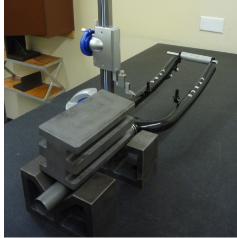
Figure 5.4: The fork of the Davis Bicycle setup for measuring the fork offset.
