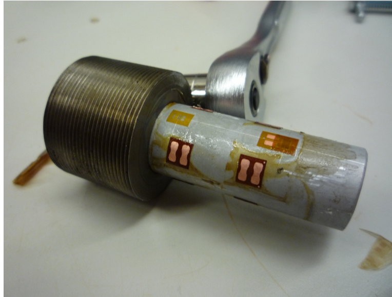
Figure 9.11: One of the foot pegs after the strain gages were applied. The 7075 aluminum peg was press fit into the bottom bracket insert made from 1018 steel.
