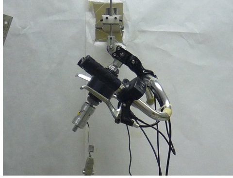
Figure 5.12: The handlebar mounted as a torsional pendulum.
