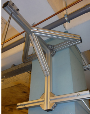
Figure 5.16: The rigid pendulum fixture from the Delft experiments mounted to a concrete column.
