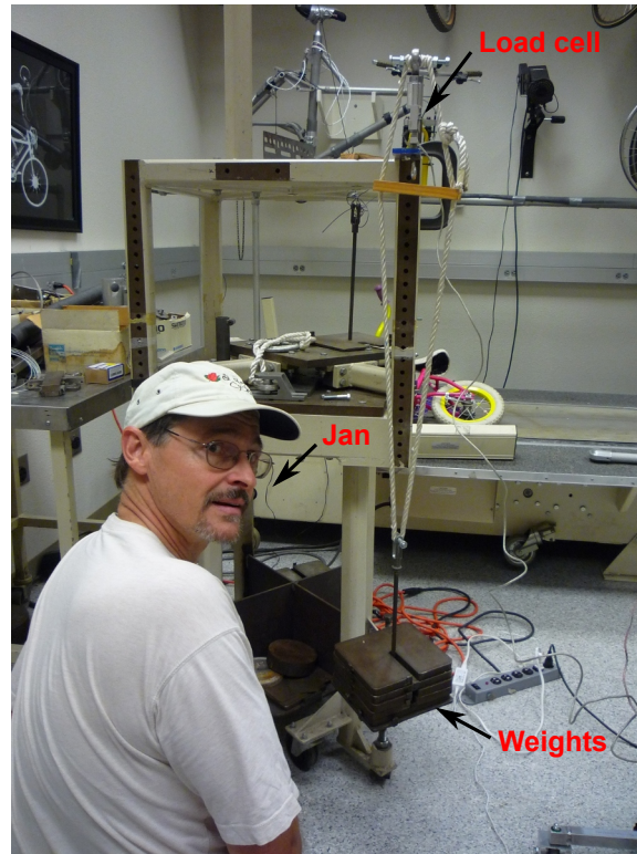
Figure 9.31: The load cell under a compressive static loading during the calibration procedure, with Jan looking on.
