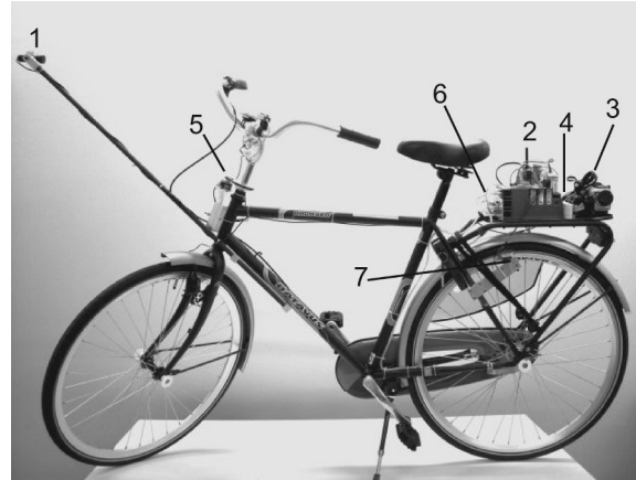
Figure 7.1: The instrumented bicycle with camera boom and video camera lens (1). On the rear rack the measurement computer (2), video camcorder (3) and battery packs (4) are positioned. Measured signals are the steer angle and steer-rate (5), rear frame lean- and yaw-rate (6) and forward speed (7).
