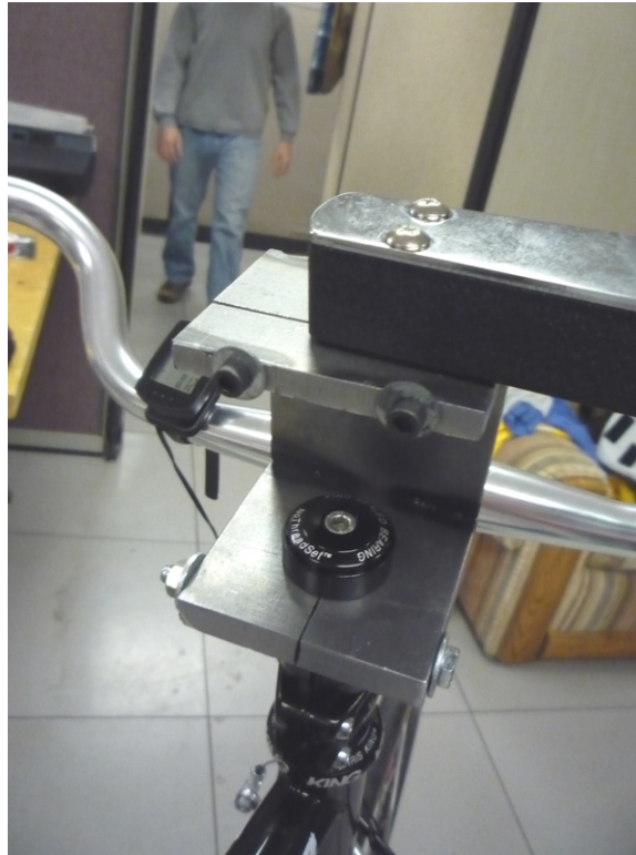
Figure 9.16: The mounting bracket for the torque wrenches. The lower portion clamps to a 1 1/8" steer tube and the upper portion clamps of a 1/4" socket end.
