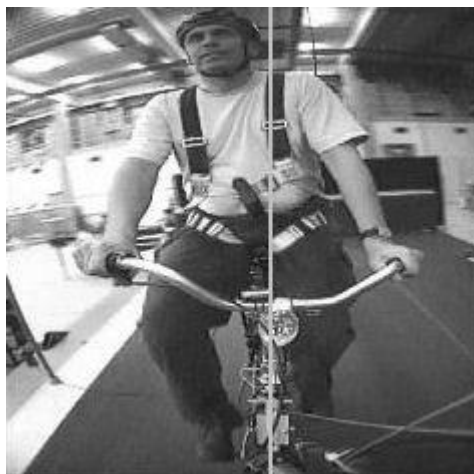
Figure 7.12: Video still directly after a perturbation (lateral force applied from the rider's right by a rope at the saddle tube) at 5 km/h. Vertical grey line indicates the bicycle mid-plane. Note the lateral right knee motion and steering action and the small upper body lean.
