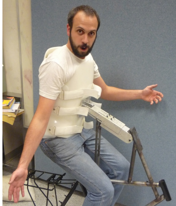
Figure 9.2: Jason strapped into the rigid rider harness. The arm allows for multiple degrees of adjustability to allow different riders and seating positions.
