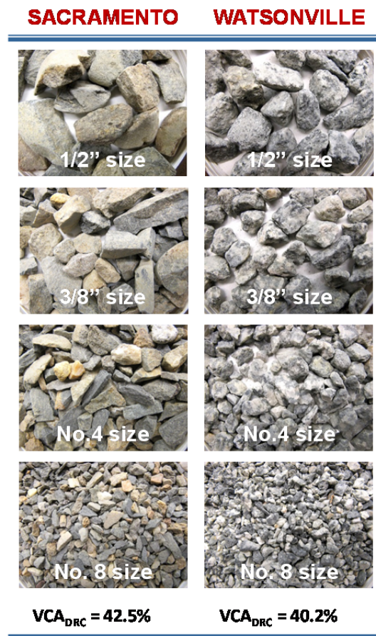
Figure 2.1: Aggregate comparison above break point sieve size. (The VCA DRC was based on 3/8 in. OGFC gradation.)
