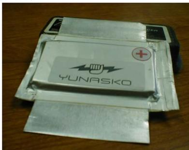
Figure 3: Photograph of the 5000F Yunasko Hybrid ultracapacitor 5000F device
