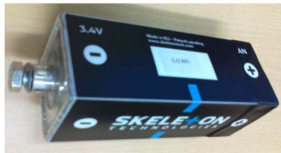
Figure 1: Photograph of the 3200F Skeleton Technologies device
